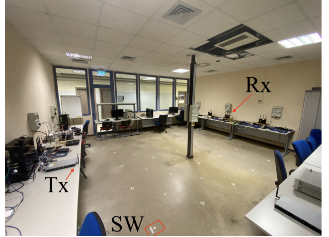
Figure 9: Photo of the laboratory described in Fig. 8, the pole in the middle with electrical outlets clearly creates a complex electromagnetic environment; the transmitter is labeled with ‘Tx’ on the west side while the receiver used in the one in the middle on the east side of the lab. Some of the \xi spots are visible on the floor (white dots) with the coordinate origin one marked ‘SW’.
