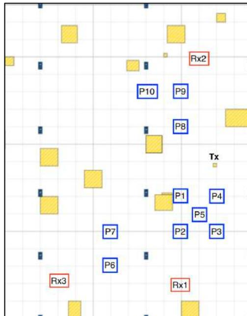
**Figure 1.2.14:** Portion of w-iLab.2 we used for the experiments with the position of the transmitter (Tx) the three receivers (Rx1,2,3) and the positions of the person (P1,...,10) used both for training and testing the localization system; the squares of the grid are 1m.
