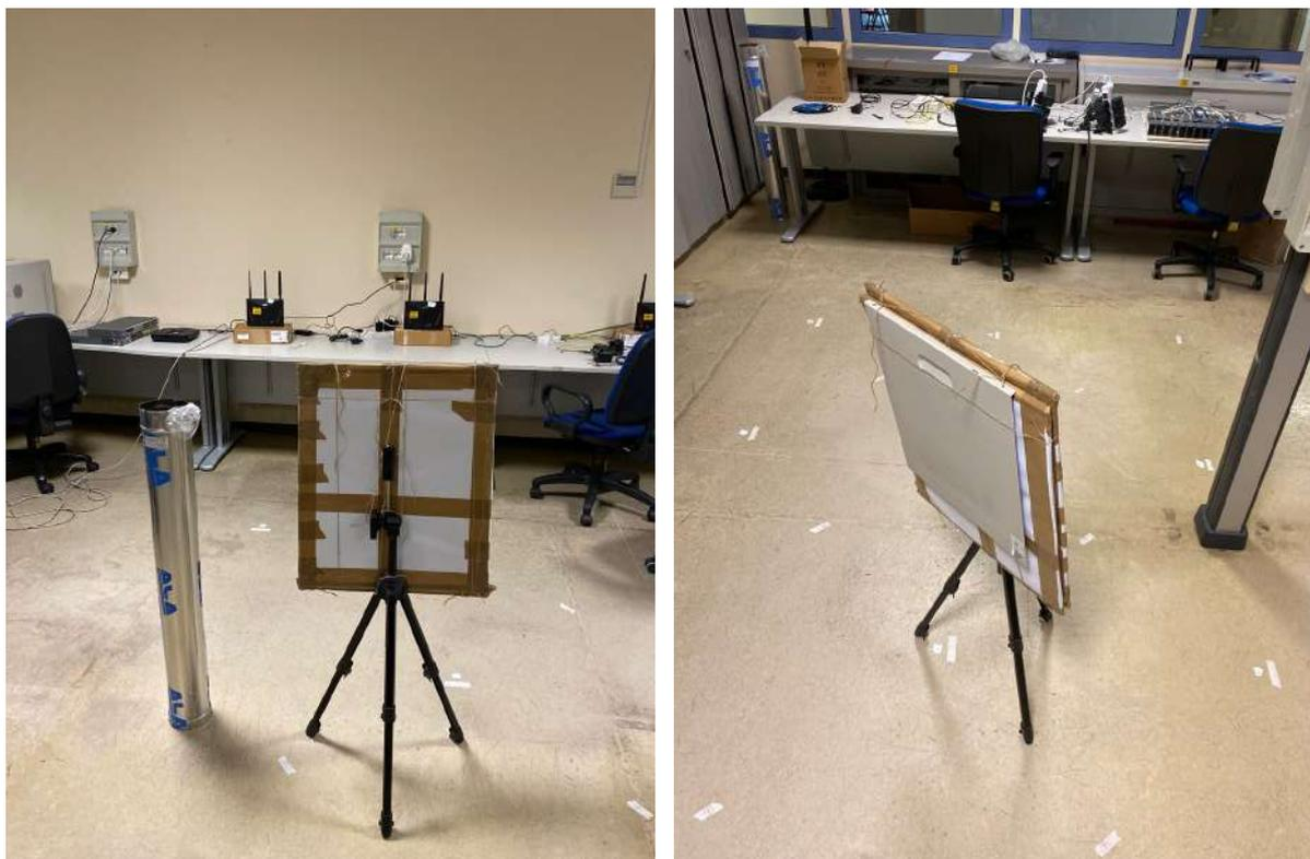
**Figure 1.2.9:** The "fake robot" (tripod with reflective panel) and the stove pipe used for localization experiments with objects.
