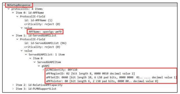
Figure 5-14: NGAP's Setup Response.
