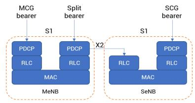
Figure 3-2: Dual connectivity with split bearer [11]
