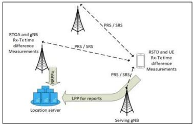
Figure 2-1: Downlink-Positioning in NR [9].
