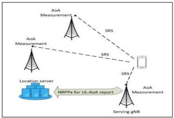
Figure 2-2: Uplink-Positioning in NR [9].
