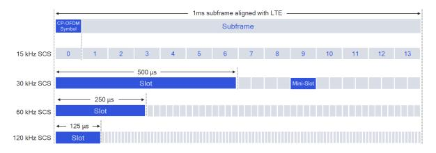
Figure 4-2: Mini slot concept, source: https://devopedia.org/5g-nr-transmission-time-interval.
