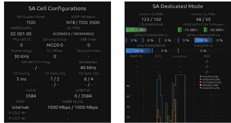
Figure 5-7:Cell configuration (Left) and Analysis about the resource blocks, QAM (Right).
