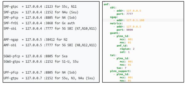
Figure 5-3: The Default Core Functions address over the same machine and the modified AMF's file.
