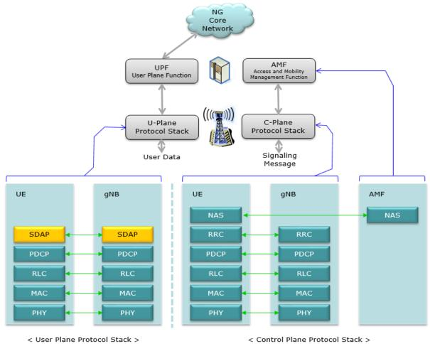
Figure 3-1: User-Plane and Control-Plane in 5G's Protocol Stack [10]
