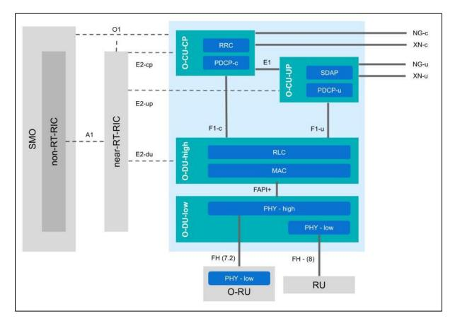
Figure 1-4: gNB high-level architecture and splits, source: https://www.srslte.com.
