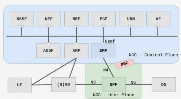
Figure 1-1: A simplified 5G Architecture with the main elements and components[3].
