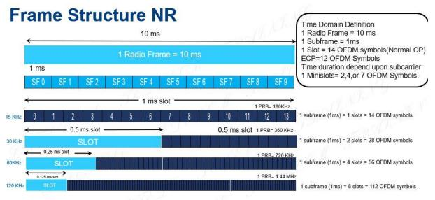
*Figure 4-1: Frames, subframes, and slots in the time domain of NR, source: https://cafetele.com/5g-nr-frame-structure.*
