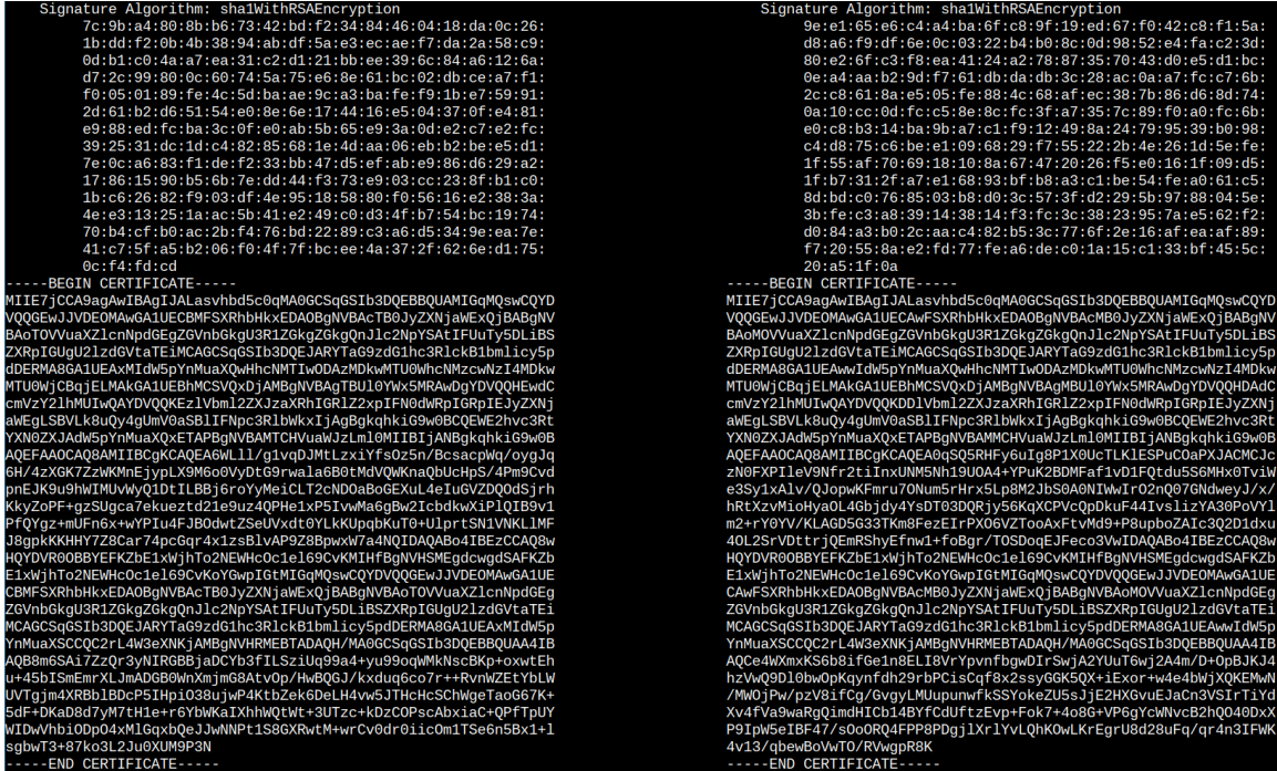
Figure 13: On the left, signature and certificate of the genuine root CA. On the right, signature and certificate of the forged one.
