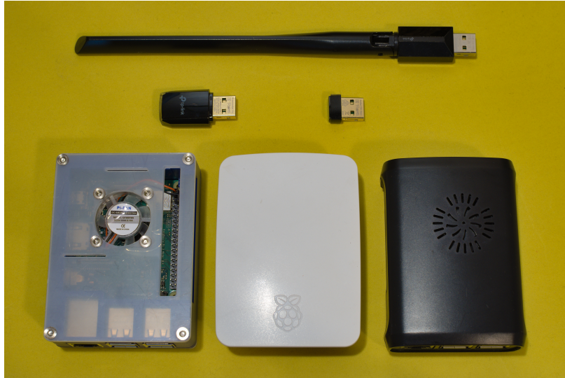
Figure 10: The three Raspberry Pi 3 model B+ along with the three different TP-Link Archer T2U dongles we used in our live test.
