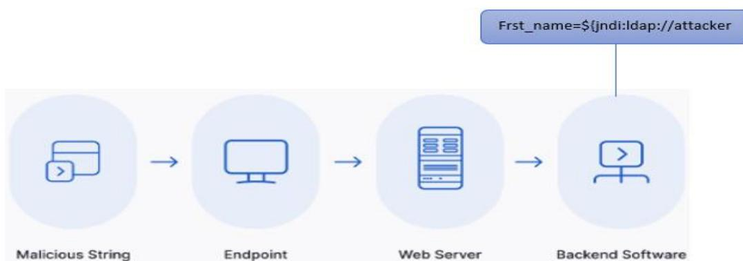
Figure 55: Malicious strings can permeate to back-end software running vulnerable Apache Log4j version.
